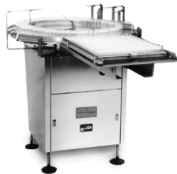
Unscramblers, Accumulators and Surge Tables
