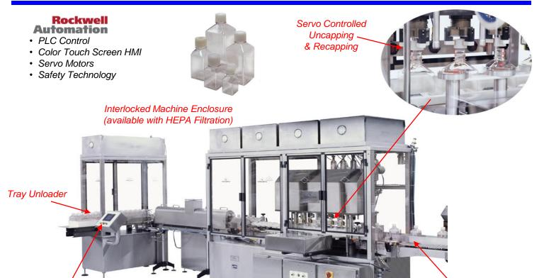
The **3600 Series** is truly unique in the industry, as we process "pre-capped" bottles! This machine performs bottle un-capping, liquid filling, and recapping of the bottle, all on a single frame!
